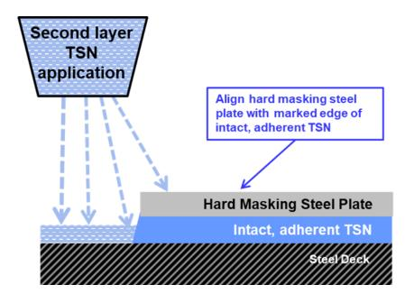
Figure C-6: Cross section view of masking alignment for second layer of TSN
