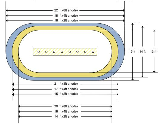
Figure D-1: Area to abrasive blast
