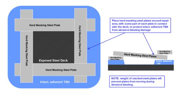
Figure C-3: Example of hard masking plate configuration around repair area
