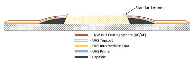
Figure E-2: Cross section of coating system and anode
