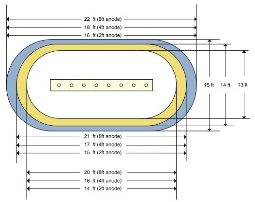
Figure E-1: Area to abrasive blast
