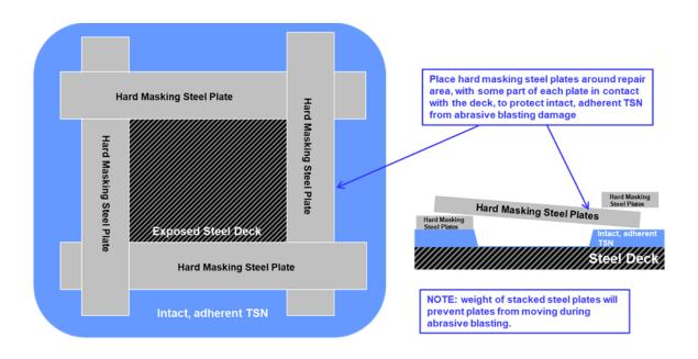
Figure D-2: Example of hard masking plate configuration around repair area
